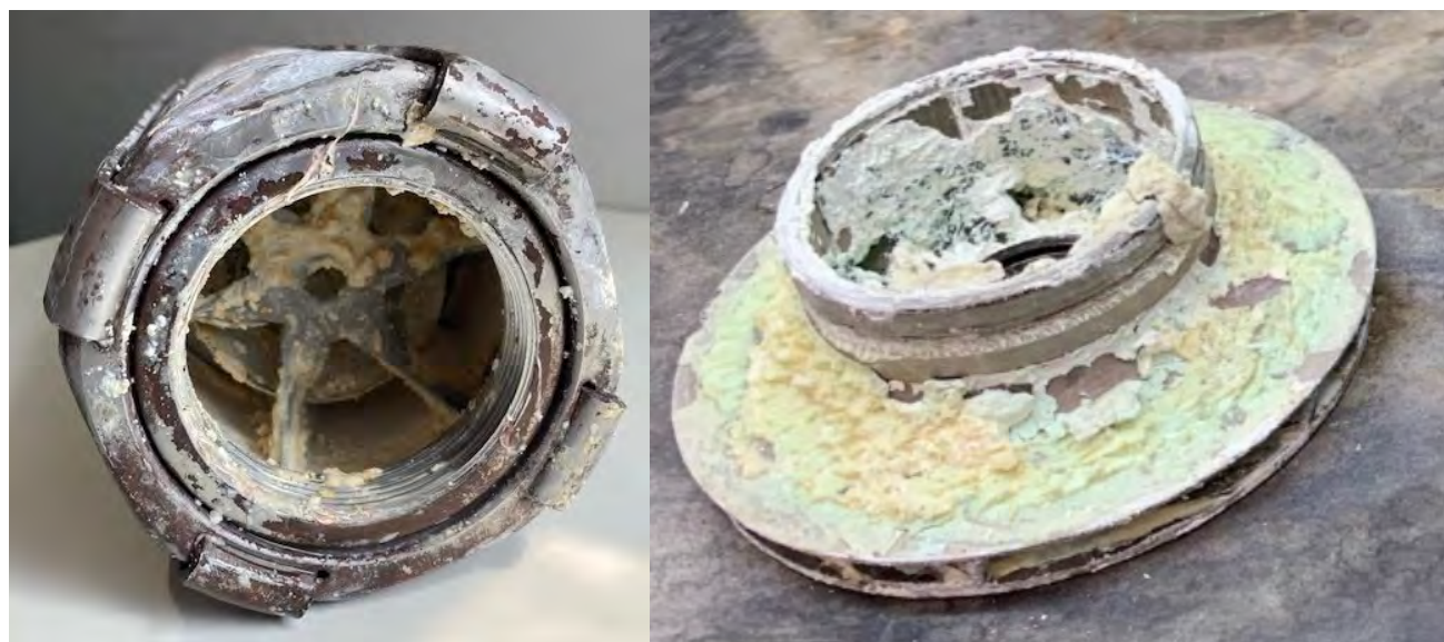
Figure 4-62 EB05 pump components. Left; inlet to foot valve. Right; one of the three impellers
