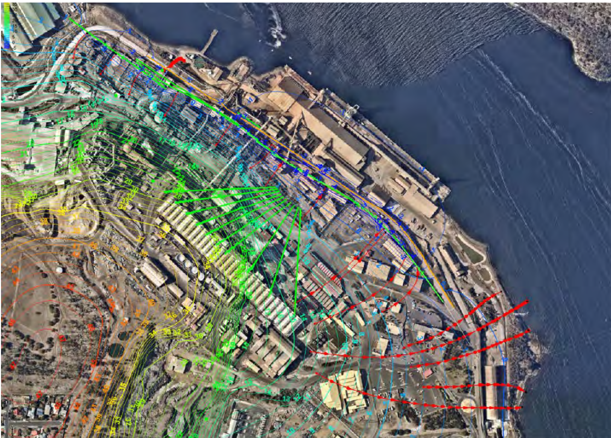
Figure 2-7 Modelled groundwater flow for the main operational area of the site with the new grout curtain and horizontal drain in place
